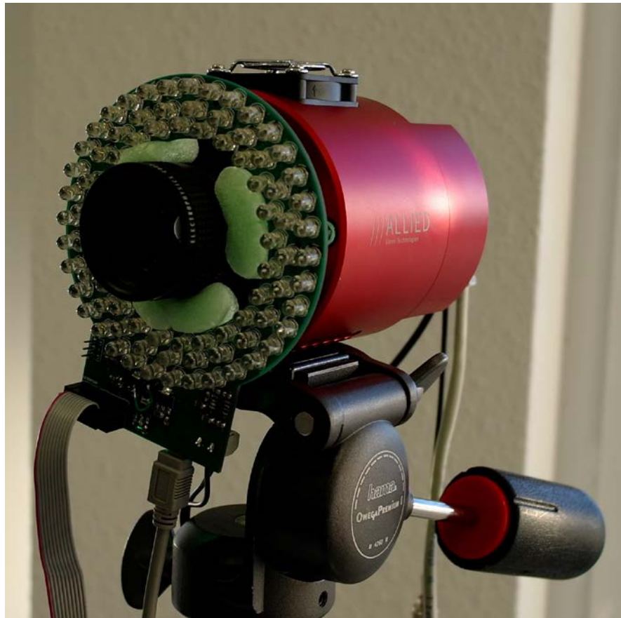
Figure 3: Setup of the camera system with attached ring flash.
